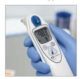
To change the temperature display, press and hold the Co/Fo button for 2 seconds when the LCD screen is active.
